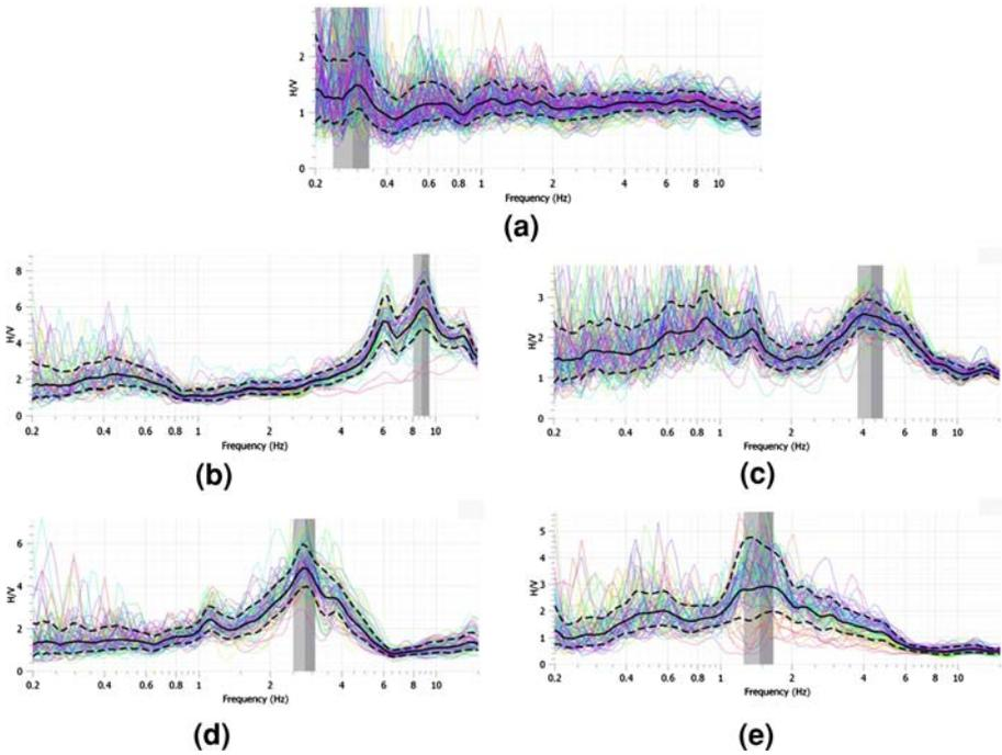
**Fig. 7** H/V spectral ratios evaluated for several RAN stations. **a** An example of H/V spectral ratio lower than 2; **b–e** H/V spectral ratio classes. The predominant frequency peaks are indicated by highlight bands
