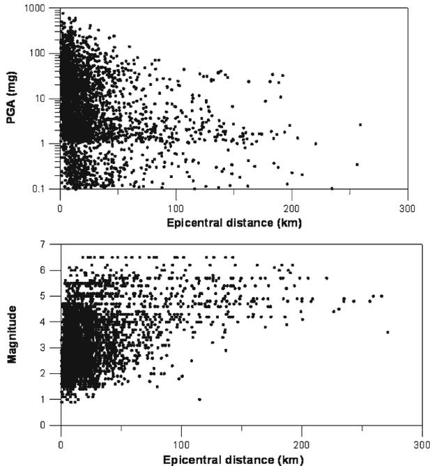
**Fig. 11** PGA (*upper part*) and magnitude (*lower part*) versus epicentral distance graphs for the RAN strong motion records
