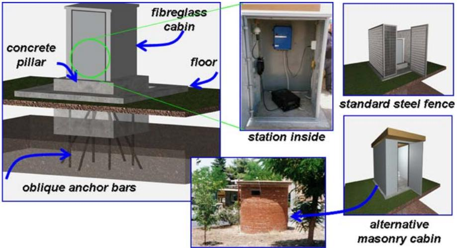
Fig. 5 Installation phases of a typical Ran digital station
