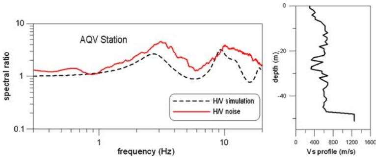
**Fig. 8** H/V spectral ratio estimates, respectively, for the AQV transfer function simulation and noise. On the *right side*, the AQV, Vs profile, applied for the 1D ground response analysis
